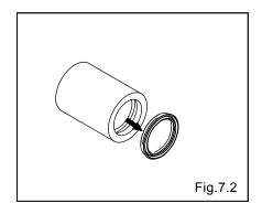
• Remove the packing from the throat bearing. [Fig.7.2]
