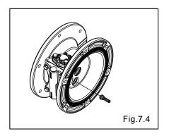
• Remove the pilot valve assembly. [Fig.7.4]
