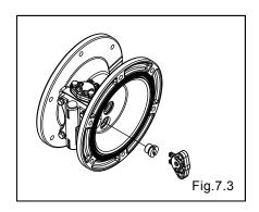
Remove the valve seat by the plate B (refer [6.1 Removal] for the plate B). [Fig.7.3]
