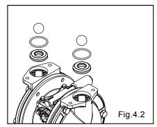
• Remove the ball, o ring, and valve seat. [Fig.4.2]
