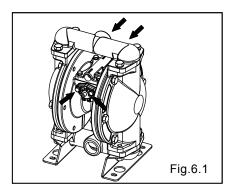
•Unscrew the four bolts and remove the plate B, the plate C and the gasket.[Fig.6.1]
