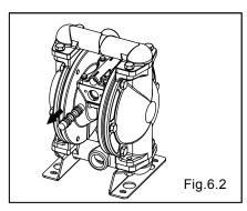
Remove the spool valve assembly, and remove the seal rings from the spool valve assembly.[Fig.6.2]
