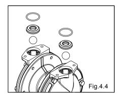
• Remove the O ring, valve seat and ball. [Fig.4.4]
